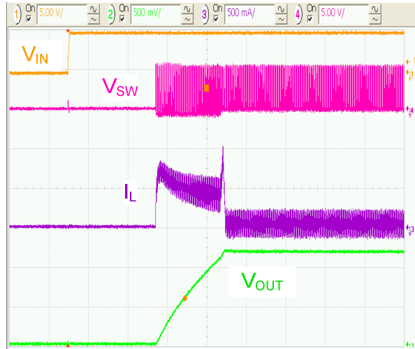
Figure 4. Startup with 100mA Resistive Load
